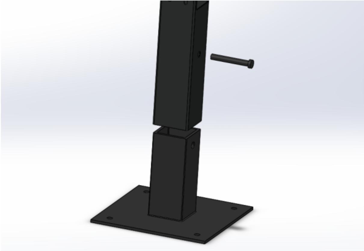
Figure 78: Exploded view Footpiece
