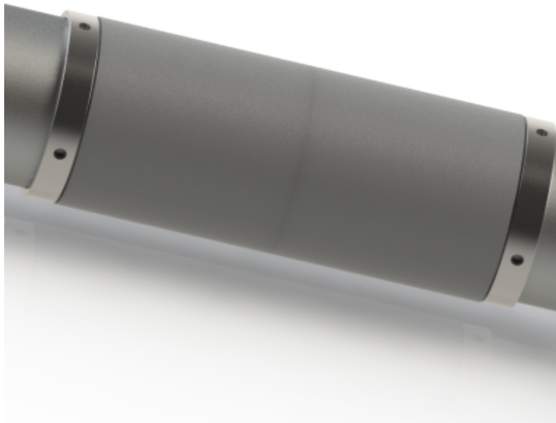
Figure 74: Collar with self-lubricating bearings
